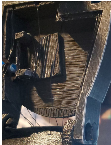
Figure 2.6.5: Tendon threading from Palm to Forearm
